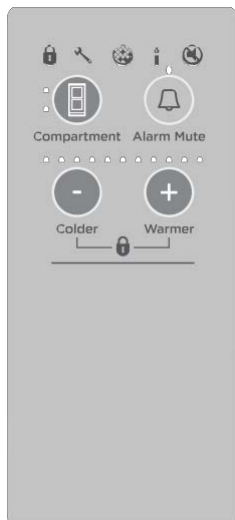
Internal control panel for Tasman models
