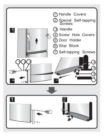
6 Loose screws used to fix the middle hinge and remove middle hinge. Then remove the lower door.
