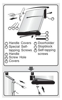
8 Change screw hole covers on middle cover plate from left to right (as shown in figure below).
