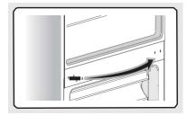
9 Place refrigerator flatwise, remove part ③ and then loose screws ④. Remove part ② and part ①.
