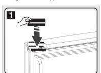
Take the reed switch out of the coping block (parts ③ and ⑥ in step 3) and mount it on another block for use (which is marked "R" in the plastic bag). Put the coping block just removed back into the plastic bag.
