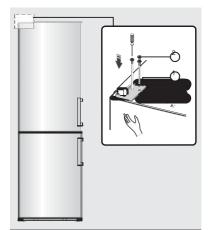
Install the upper hinge cover (which is in the plastic bag).
