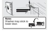
13 Screw out the upper hinge axis, turn the upper hinge over and fix axis on it. Then place it at side for use.
